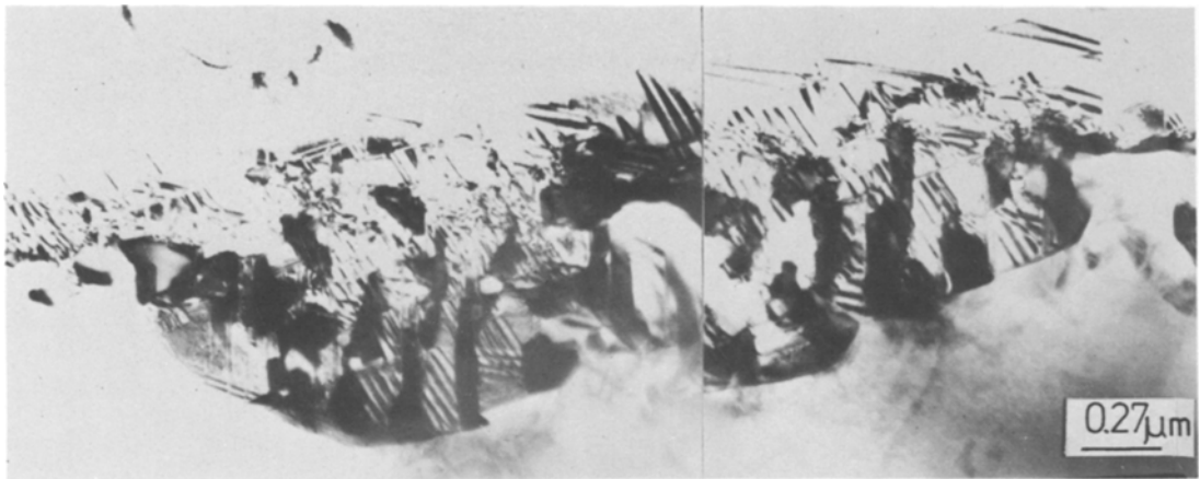
Figure 16 Aged at 760° C for 5 h. TEM picture of lamellar precipitation and stacking faults at grain boundary. Note bowing out of lamellar region into neighbouring grain.
